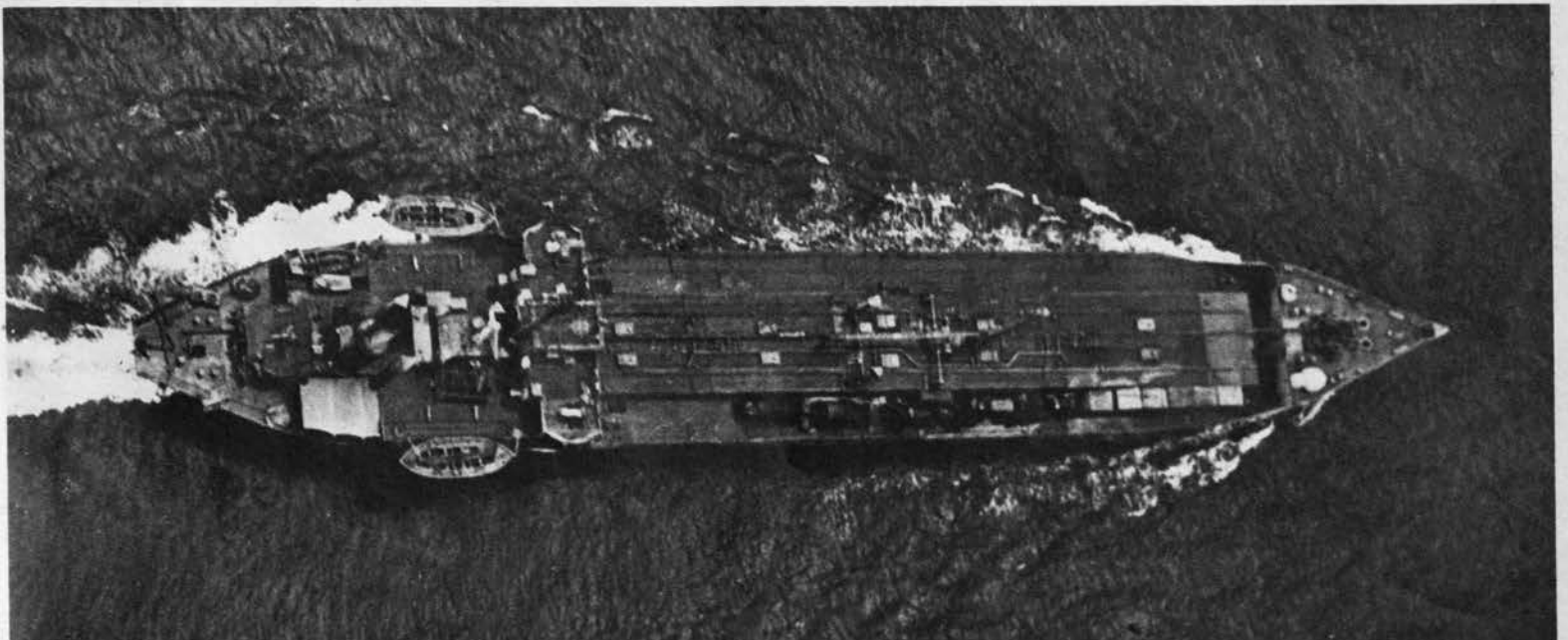
"Economy" hull , with sharply angled bow, narrow tapering stern, stands out in this view of Sugar Able Sugar. Note pairs of small vent
